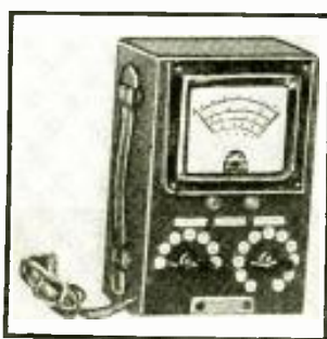
Volt-ohm-current meter. A power level scale directly in db. is included for power measurements. (1417)
