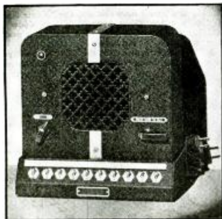
Selective-type interphone. Note:—Toggle switches permit simultaneously tying-in 4 stations. (1390)
